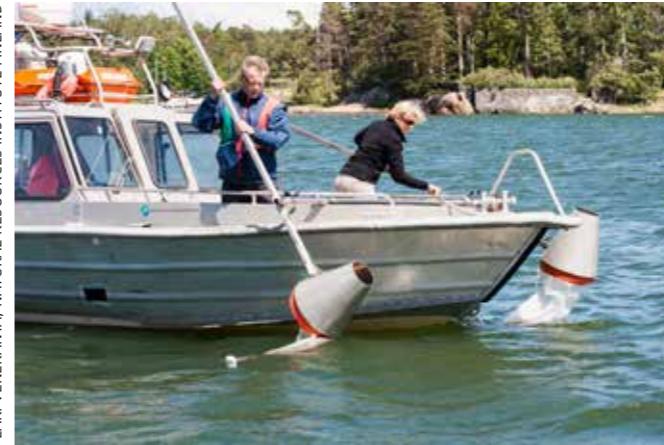
Fish breeding grounds are surveyed in open waters using Gulf ichthyoplankton samplers.
